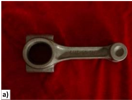
Fig. 25. (a) Engine connecting rod; (b) Engine intake valves, both made of DRTCs. Pictures courtesy of Central South University. (For interpretation of the references to colour in this figure legend, the reader is referred to the web version of this article.)
