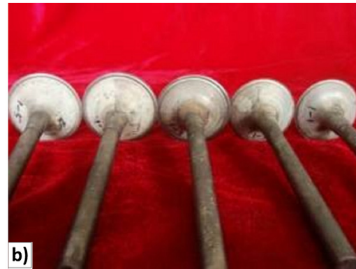
Fig. 25. (a) Engine connecting rod; (b) Engine intake valves, both made of DRTCs. Pictures courtesy of Central South University. (For interpretation of the references to colour in this figure legend, the reader is referred to the web version of this article.)
