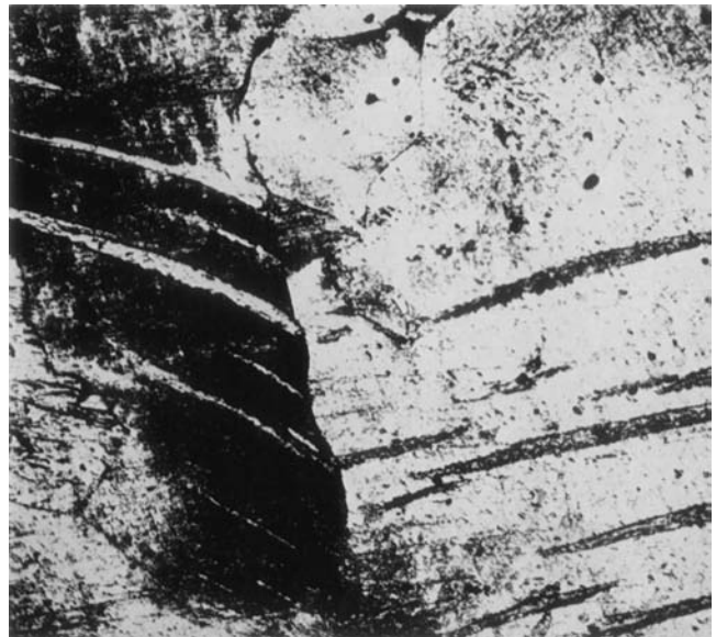
Fig. 4—Deformation bands in a transverse section of polycrystalline iron wire reduced 30 pct by drawing. Dilute nitric etch. Magnification 100 times (Fig. 3 from Barrett and Levenson [28] ).
