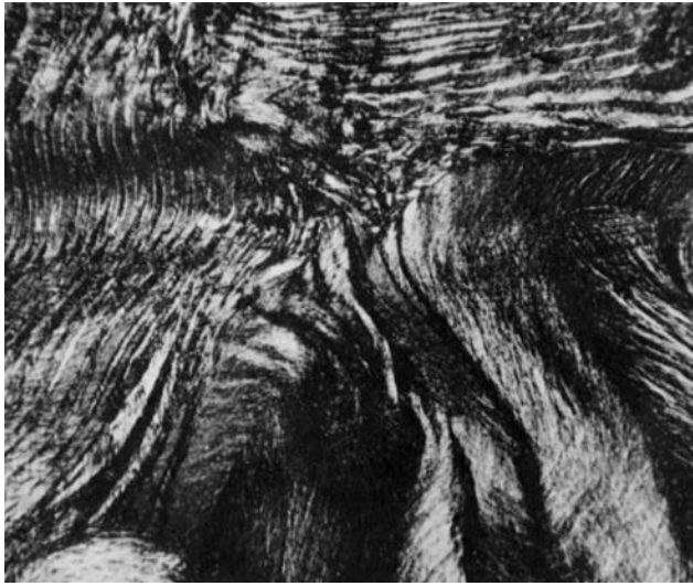
Fig. 5—Etched transverse cross section of an aluminum rod extruded 90 pct at 77 K from a \langle 111 \rangle single crystal revealing DBs in polarized light. Magnification 45 times (Fig. 7 from Reed and McHargue [47] ).
